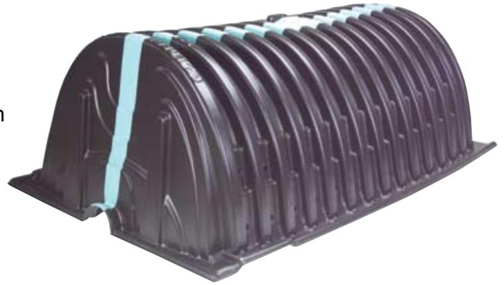
Engineers from Phoenix-based Evans Kuhn and Associates, Inc. specified a CULTEC two-tiered subsurface retention system to capture, treat and retain run-off until it could be displaced. The system included approximately 2,400 Recharger® 330 HD chambers constructed of high-density polyethylene, designed to maintain a significant permanent pool of water between precipitation events.
